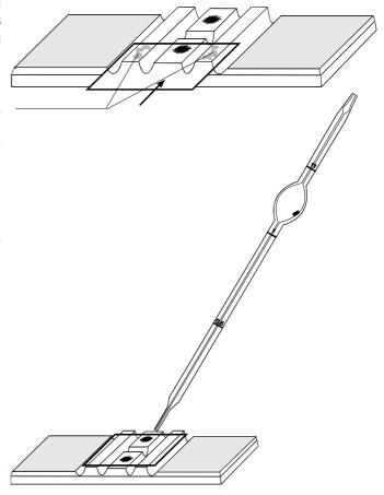
pipette must be removed. If any air bubbles are visible or if the liquid has overflown over the edges into the grooves, the chamber should be cleaned and feeding be started again.
